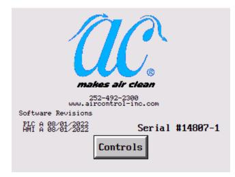
This screen is the first screen that comes up on the touchscreen controller when the hood is powered up. It lists the benches serial number, as well as the software revisions of the operating software.
